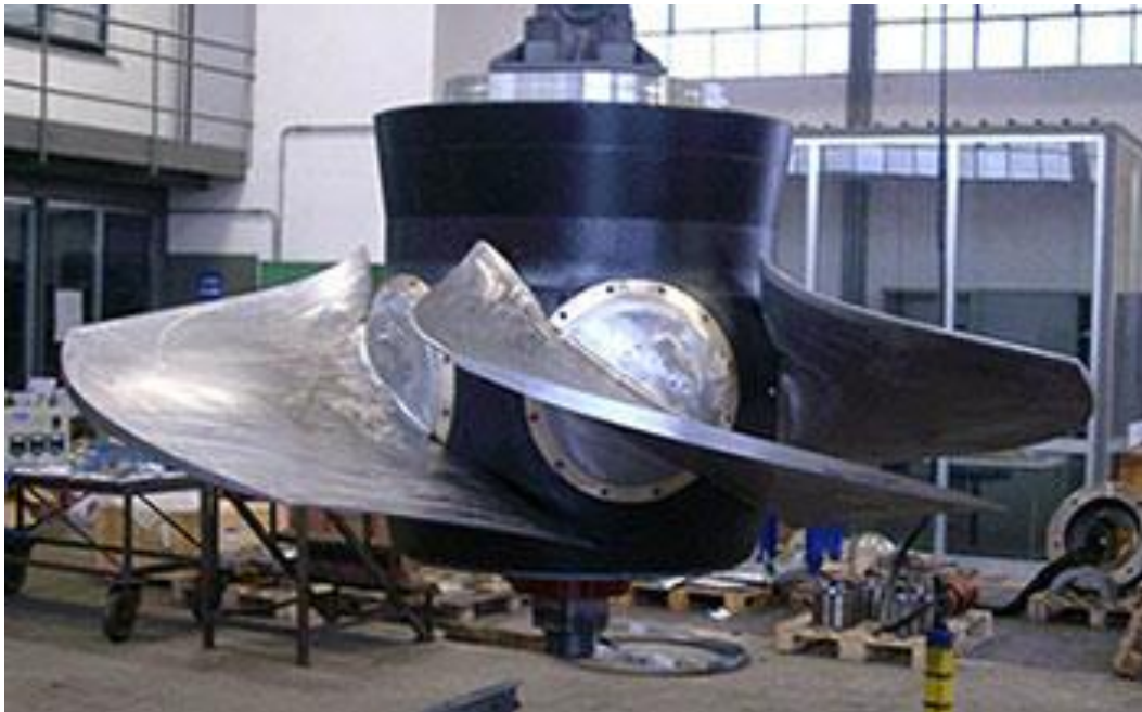
Figure 19 - Kaplan Turbine Rotor 41
