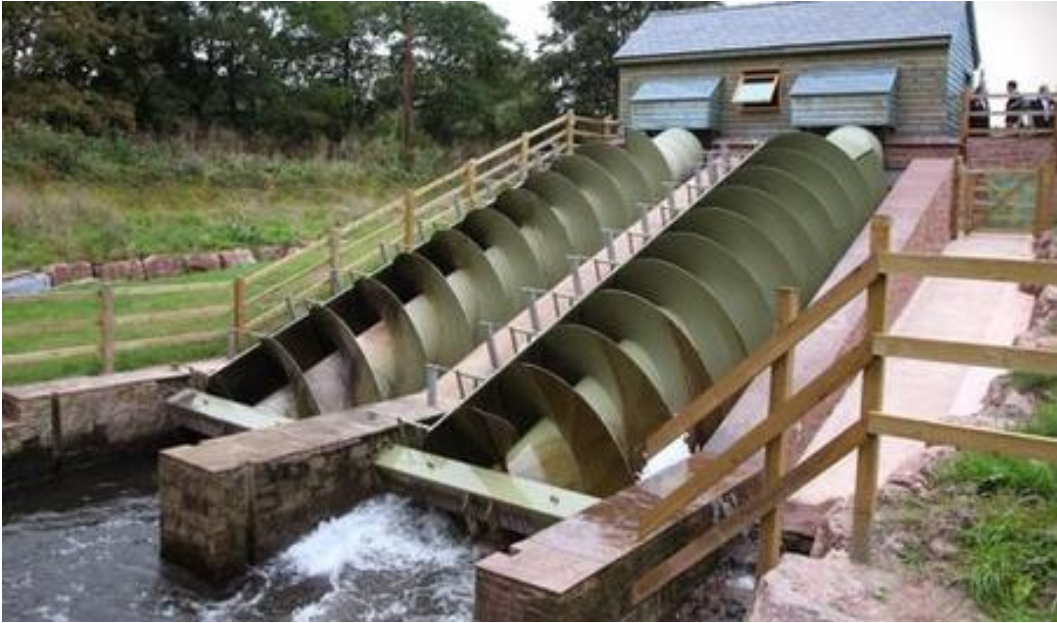
Figure 13 - Two 75kW Archimedes screw turbines, Monmouth, Wales 36
